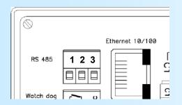
The pin (3) is Not connected
