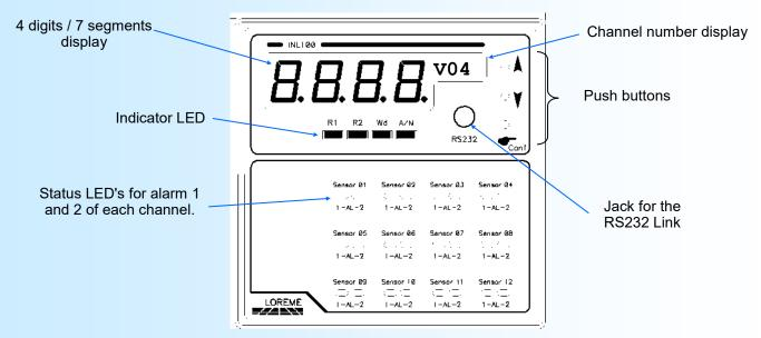
The device front panel is composed of:
