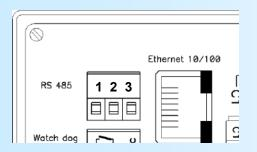
The pin (3) is Not connected
